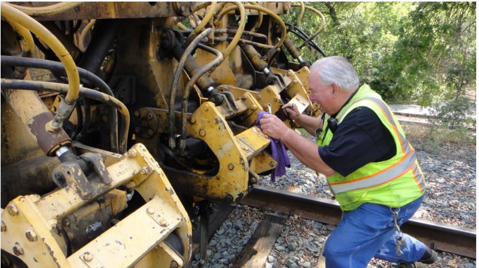
Harry is Johnny-on-the-spot making repairs to one of the vibrator motor on the old-old tamper.
